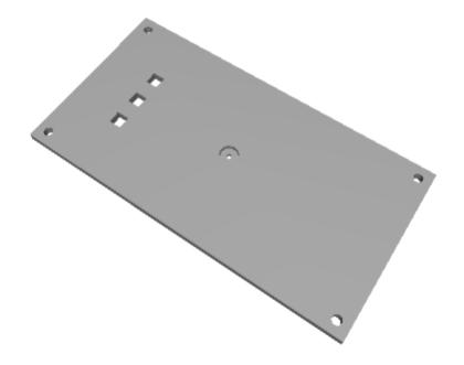
Fig. 12. Lid design for the Precision Controller enclosure.
