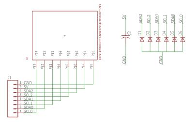
Fig. 8. Schematic of the small circuit board in the main controller, containing connections for the IMUs and also the clipping diodes for the data lines
