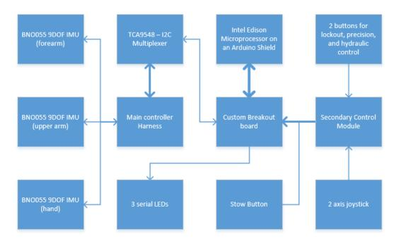
Fig. 5. flowchart showing all of the electronic hardware components and interconnections
