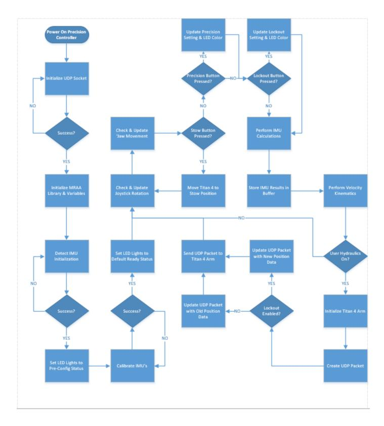
Fig. 10. Software flowchart for the Precision Controller.
