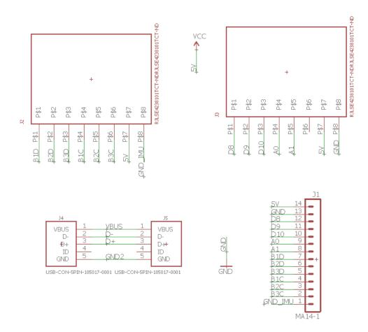
Fig. 7. Schematic of the connector board inside the enclosure, provides connection to the main controller and remote unit from the Edison through the 14 pin header
