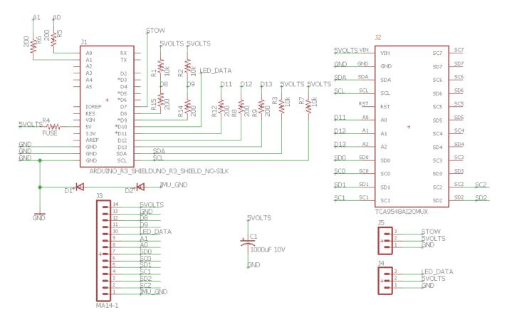
Fig. 6. Schematic of the main breakout board, connected directly to the arduino shield
