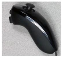
Figure A-2: The offhand module for the precision controller.
