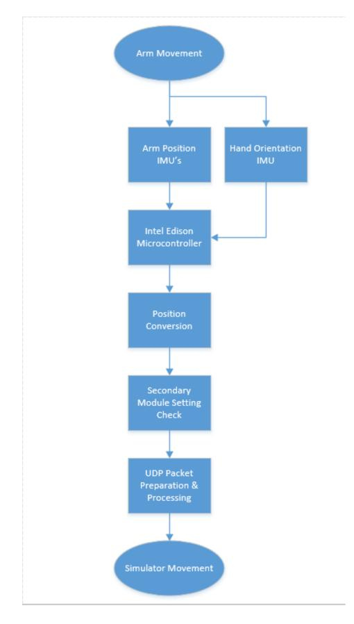
Fig. 9. Software block diagram for Precision Controller.
